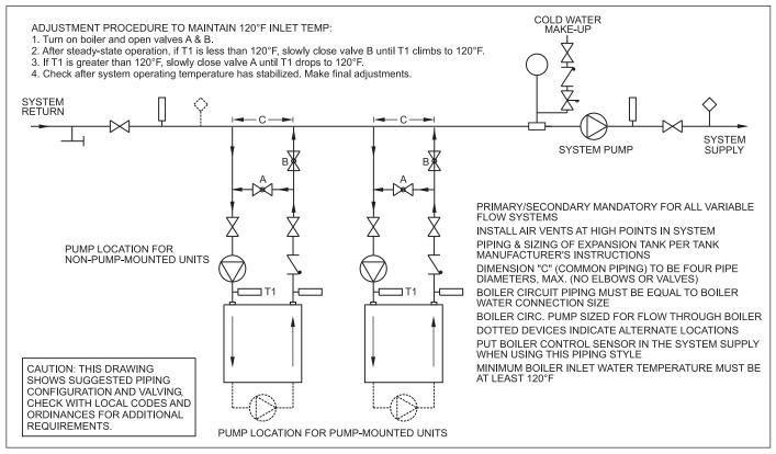
Figure 7. Hydronic Piping — Multiple Boilers, Low Temperature System.
